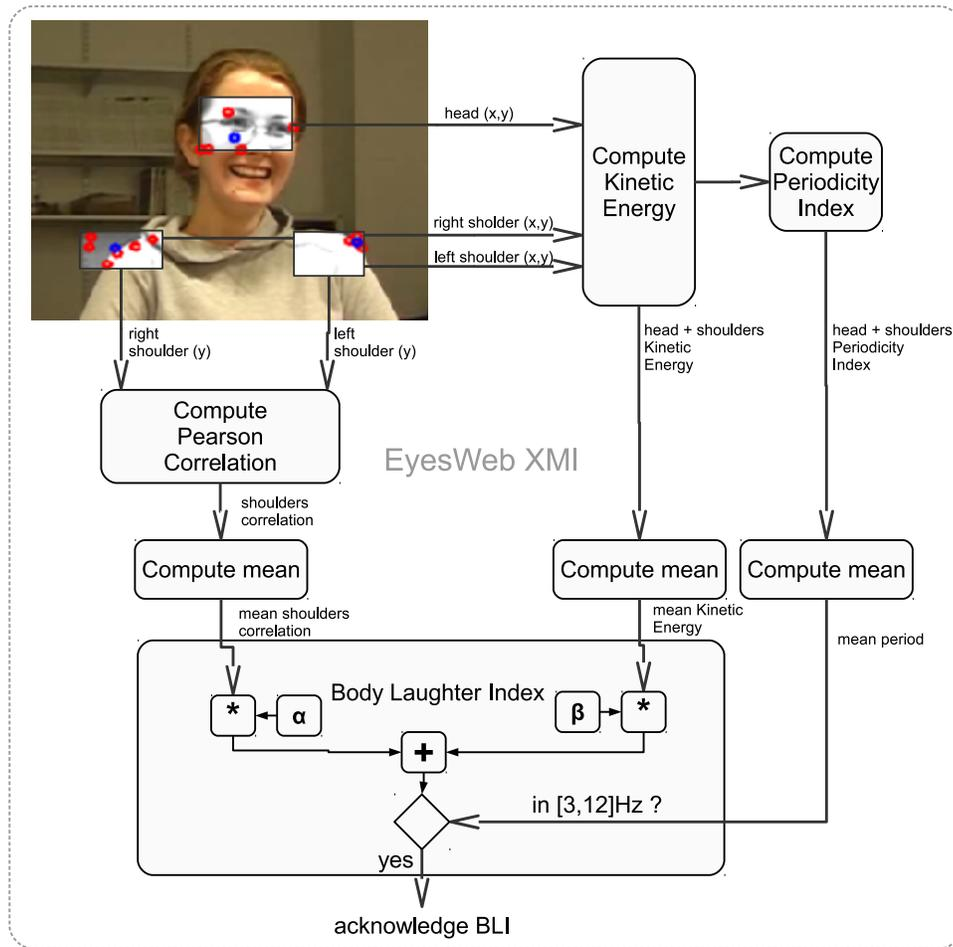
**Fig. 1.** The software architecture for computing BLI. Firstly, tracking of head and shoulders is carried out: the cloud of red points determines the Regions Of Interest (ROIs) head and shoulders are located in. The blue dots are the geometrical barycenters of each cloud. The boxes are the major software modules extracting and processing movements descriptors.
